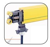
• Bumper commanding instant stop of the robot if contact with an obstacle occurs
