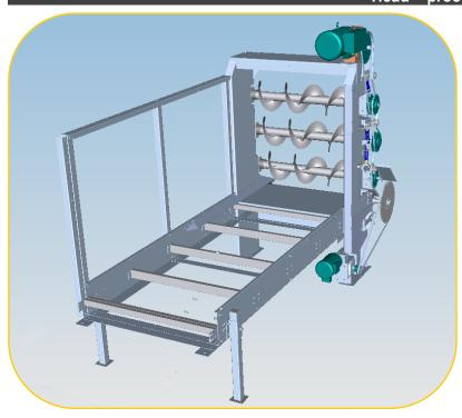
Three auger drive, designed specifically to perform "bales to bulk" (flat silos)
