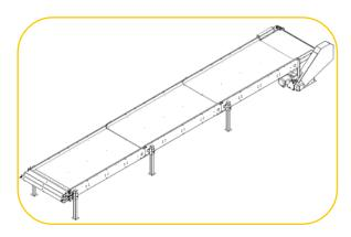
Powerful conveyor base equipped with paddle stats acting mobile deck steel, capable of operating forward – reverse.
